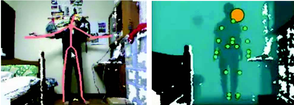
Figure 2. With the data retrieved by Kinect sensor, the program overlays a skeleton on the 3D image and tracks body joint.
