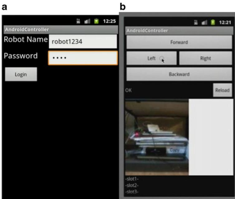
**Figure 5** Controller Graphical Interface; (a) Login Screen; (b) Robot Control Panel.
